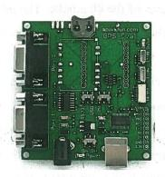
Johns Connor uses the FV-M8 32 channel San Jose Navigation GPS receiver, which supports WAAS. It is accurate to 3.3 meters and is used at a baud rate of 38400 bps. The GPS is connected to the GPS Evaluation Board from SparkFun Electronics. This evaluation board is specifically designed to work with our GPS. It interfaces to the computer through a USB port. The board converts serial data to NMEA sentences.
